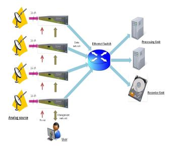
A new concept developed based on fully independent and versatile data-acquisition front-end with embedded FPGA processing capabilities. Front-end can be an industrial PC , with latest FPGA PCI Express form factor card, programmable at a higher level rather than HDL.
